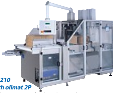
oli 210 with olimat 1 Fully-automatic final packaging line (up to 20 cases/min)
